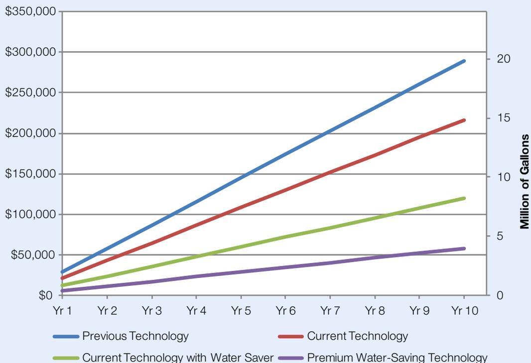
\* Previous technology vs Premium Water-Saving Technology. Cumulative washer and sterilizer consumption based on processing instrument sets for a typical 10 OR facility 260 days/year.
